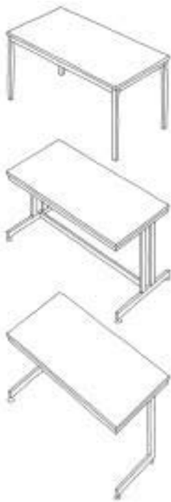
▲ FIGURE 4.1 Specialist table underframes: standard four-legged frame, 'I' frame and cantilever 'C' frame
