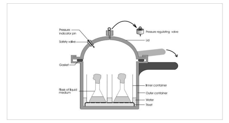
Lid with a mechanism for holding it in place. The lid cannot be accidentally released while the autoclave contents are under high pressure. Lids retained by wing nuts have two of them held on the lid, so the lid must be pulled partly open before these nuts are released.
