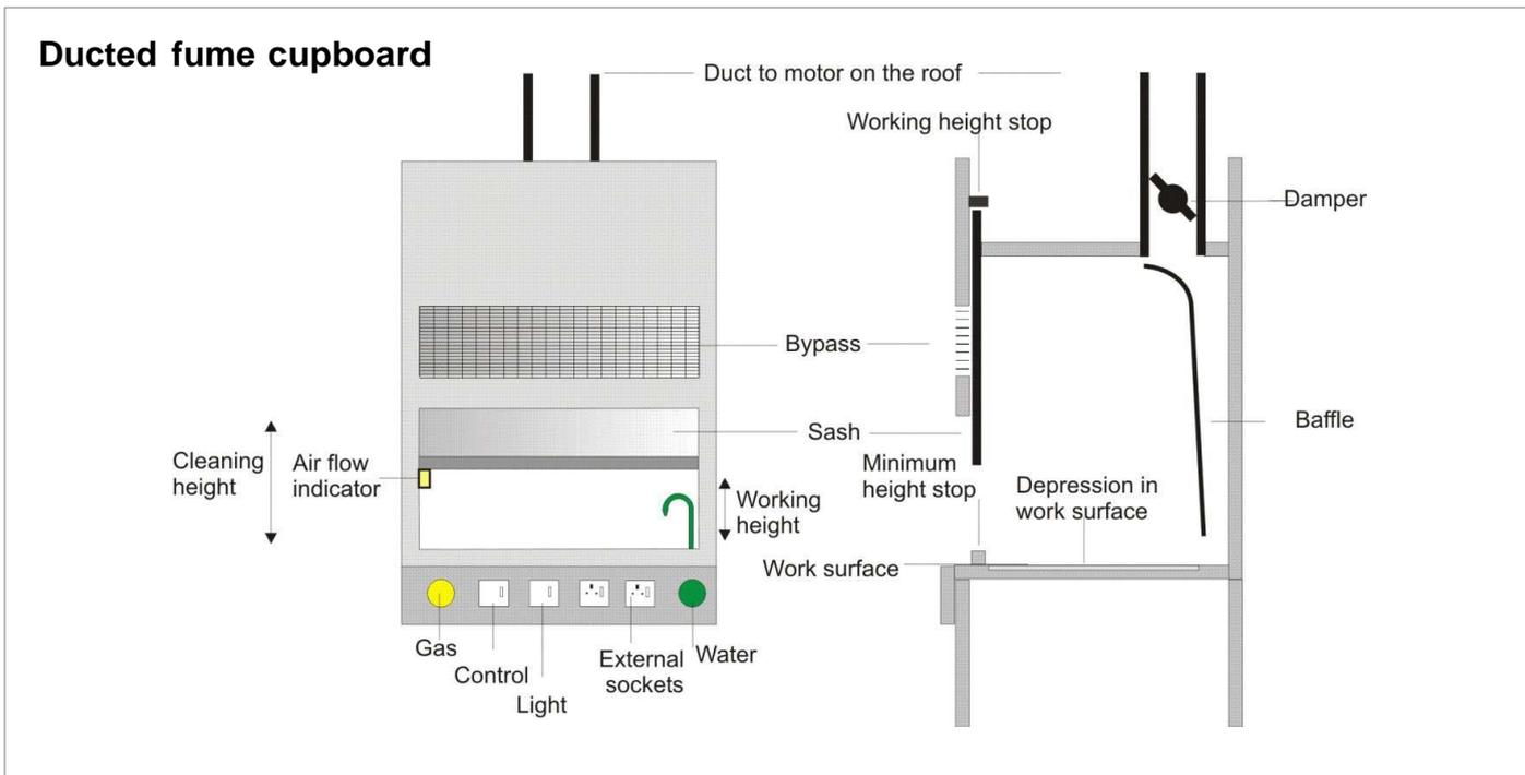
The **damper** is used when the fume cupboard is installed and commissioned to adjust the airflow to give a suitable face velocity. It should then be locked in position.
