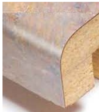
Laminate on chipboard base with a post-formed edge
