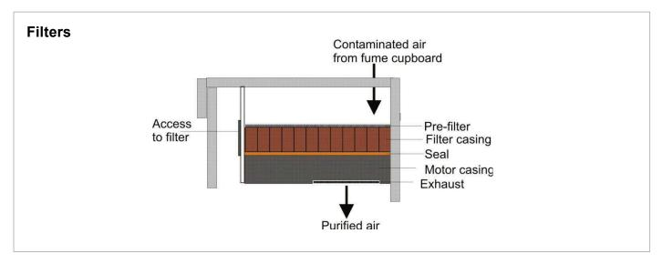
Carbon filters absorb organic vapours; in school they also need to absorb toxic and corrosive chemicals such as chlorine, sulfur dioxide, and ammonia. This is achieved by doping the carbon with, for example, sodium hydroxide to absorb acid gases, and phosphoric acid to absorb alkaline gases. Schools must ensure that educational filters are specified both initially and in subsequent replacement.
