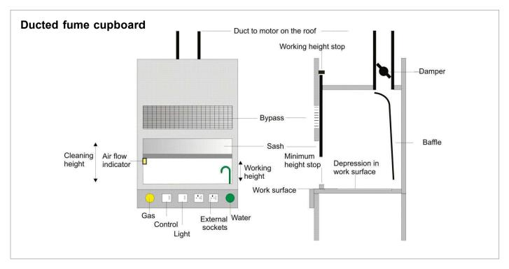
The damper is used when the fume cupboard is installed and commissioned to adjust the airflow to give a suitable face velocity. It should then be locked in position.
