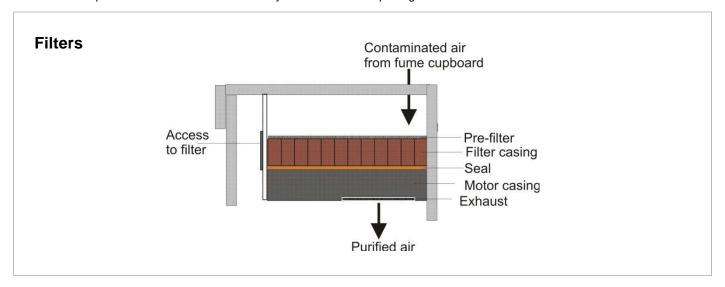
Carbon filters absorb organic vapours; in school they also need to absorb toxic and corrosive inorganic chemicals such as chlorine, sulfur dioxide, and ammonia. This is achieved by doping the carbon with, for example, sodium hydroxide to absorb acid gases, and phosphoric acid to absorb alkaline gases. Schools must ensure that educational filters are specified both initially and in subsequent replacement.
