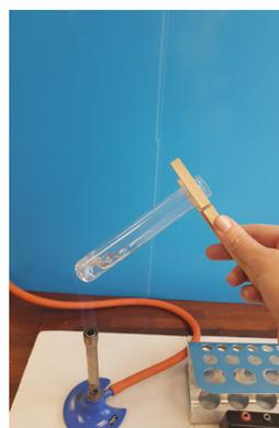
Fig.2 Keep the test tube at an angle.
